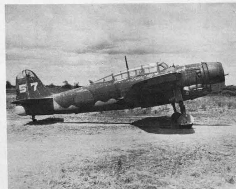
JUDY 33 Except for the nose and airscoop, both Judys are identical. Wing is low mid with slight dihedral. The greenhouse is long and low with a gradual slope down to the rear.
